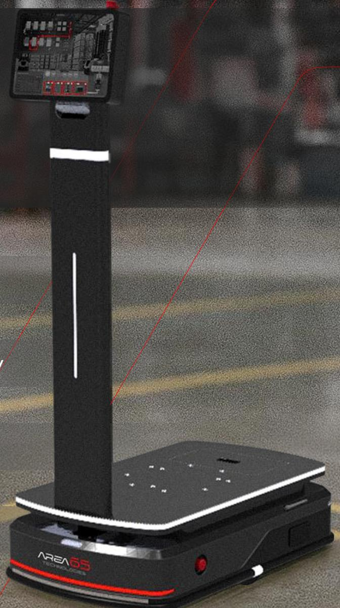
AMR-E300 is a collaborative robot engineered to automate material transport and replace manual handling on the factory floor. Equipped with an advanced autonomous navigation system, it intelligently detects and avoids obstacles, moves freely without floor markers, and operates continuously for seamless, uninterrupted productivity.
